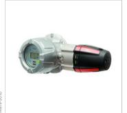
The Dräger Polytron® 5700 IR is a cost effective explosion-proof transmitter for the detection of flammable gases in the lower explosive limit (LEL). It uses a high performance infrared Dräger PIR 7000 sensor that will quickly detect most common hydrocarbon gases. A 3-wire 4 to 20-mA analogue output with relays makes it compatible with most control systems.
