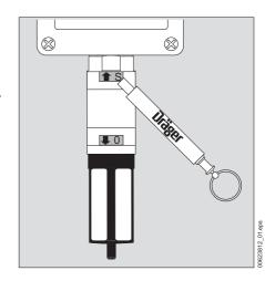
Remove the magnetic pin. The gas transmitter changes to an output signal which displays the currently set gas category according to the following table:
