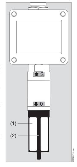
The splash guard is held by a fixture provided with screw-thread, which is also used as calibration adapter.
