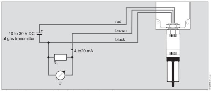
Colour code of connecting terminals and/or leads at the gas transmitter:
